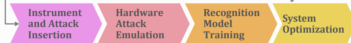
The characterization tool modifies the target design and emulates the effects of attacks against the device. Data is collected to build attack recognition models that can be used to mitigate attacks in real-time.
