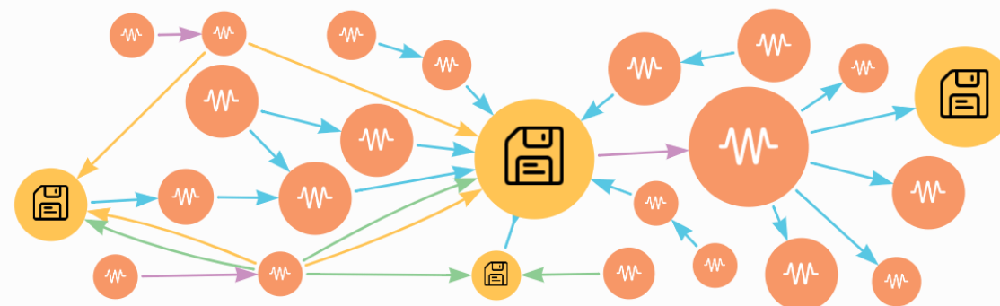
A novel influence graph structure is used to model the interactions between signals within a device. Different-colored nodes represent types of elements, and different-colored arrows signify varieties of relationships.
