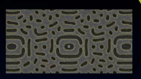
Multi-beam mask writing enables curvilinear masks for most advanced lithography
