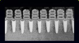
Gate all-around transistors trigger new extraction requirements and physical failure modes
