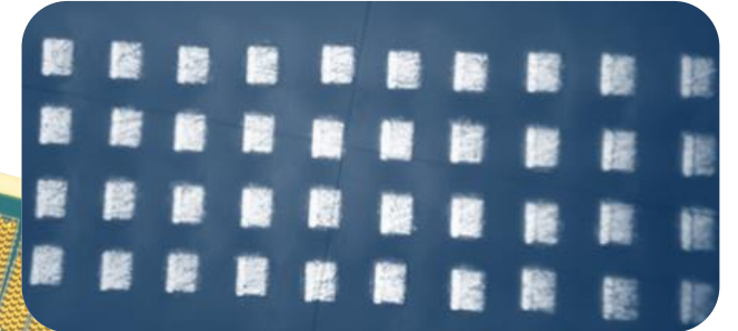
40µm pitch MEMS probe tip grid array
