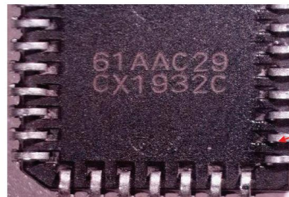
Backside, look at the black shiny paint like substance in the lower right side, the mold pin cavity is almost gone, look at the bent leads, looks like it may have been painted over to hide sanding marks and then fraudulently remarked
