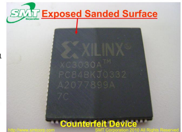
Backside, look at the black shiny paint like substance in the lower right side, the mold pin cavity is almost gone, look at the bent leads, looks like it may have been painted over to hide sanding marks and then fraudulently remarked
