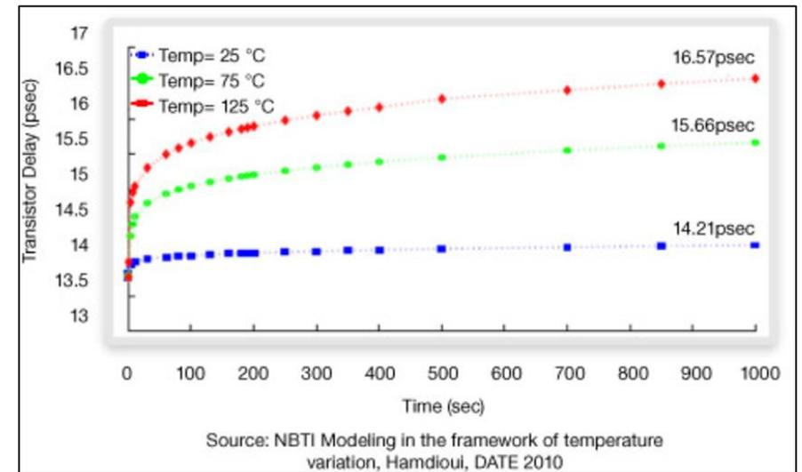
Aging impact on transistor delay
