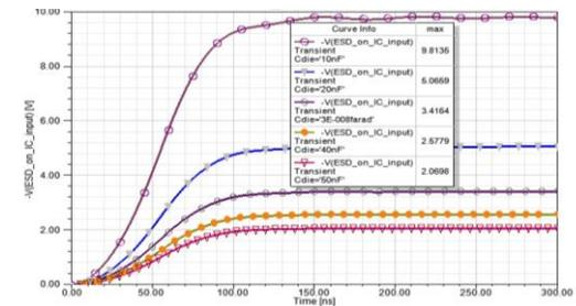
**Chip pin V(t) for different CECM. Higher Cdie results in lower pin residual voltage**
