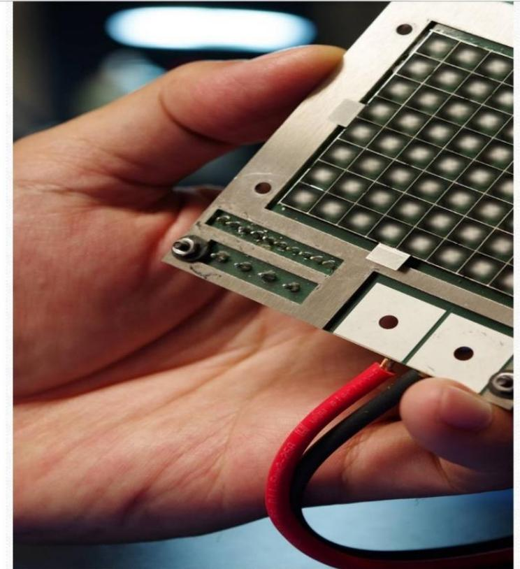
**Figure 4** The original Movandi BeamX prototype is a 64-element phased array antenna based on bulk CMOS processes. Image courtesy of Movandi Corporation.
