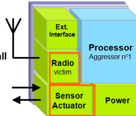
Coupling Noise from switching digital to sensitive analog through the silicon
