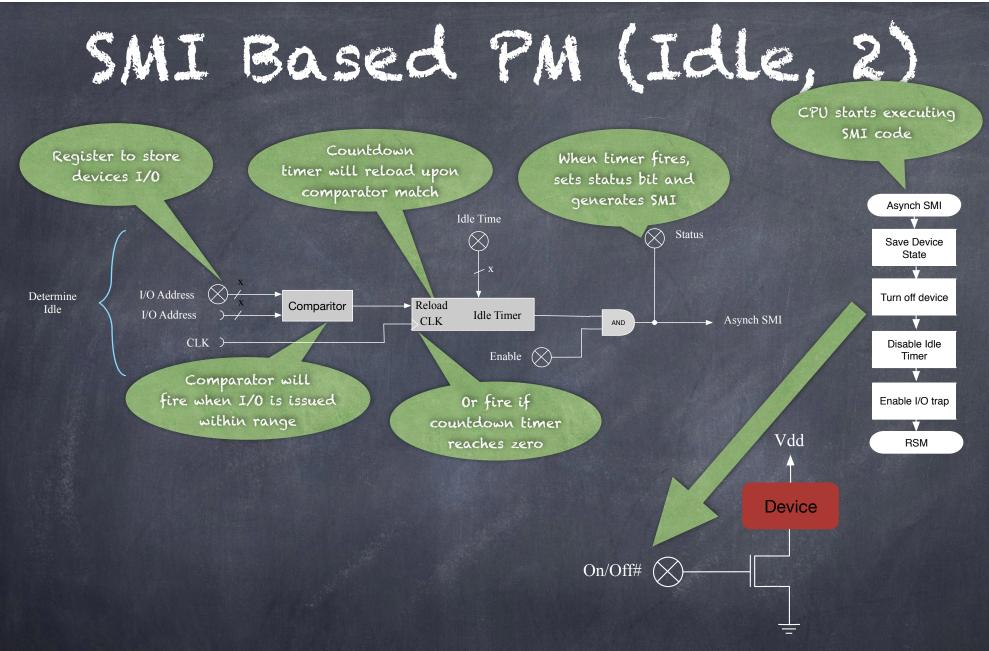
Seach device would have a set of "shadow registers" with a timer. The notebook would enable an idle time, and when this expired the device would be turned off
