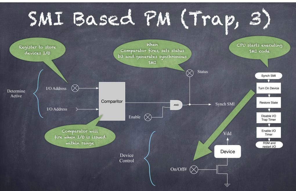
For activity its the reverse, a match to the I/O address would fire an synch SMI which would turn on the device, restore its context, and then re-start the I/O access after the RSM instruction.
