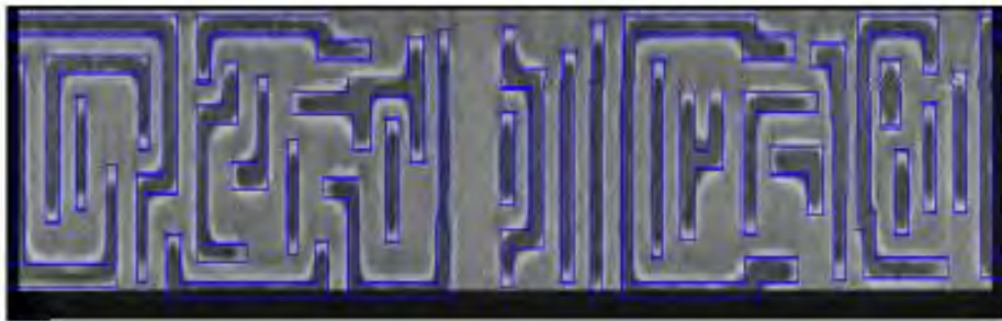
14nm node ARM M1 clip, 46nm minimum pitch, exposed on an NXE:3300B with conventional illumination
