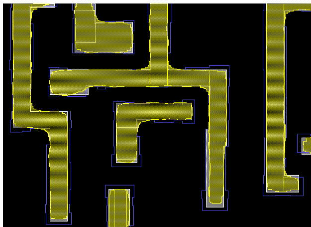
Figure 3: Lithography Variation. White - Original Drawn. Green - Manufactured. Blue – Corrected Drawn
