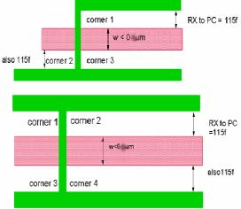
E.g. 115f PC inside corner\* to (GATE not DECAP), for device width < 0.xx um and (GATE not DECAP) neighbored by more than 2 PC corners\* [115f value determined from minimum device width of 0.yy um. For device width RX >= 0.qq um follow rule 115dd] >= 0.zz.
