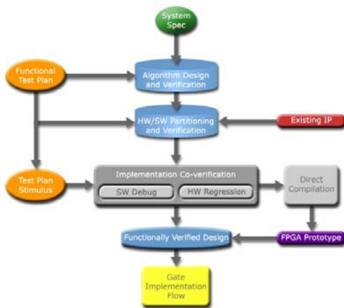
Figure 3: The SCSD methodology supports a specification-driven system verification design flow
