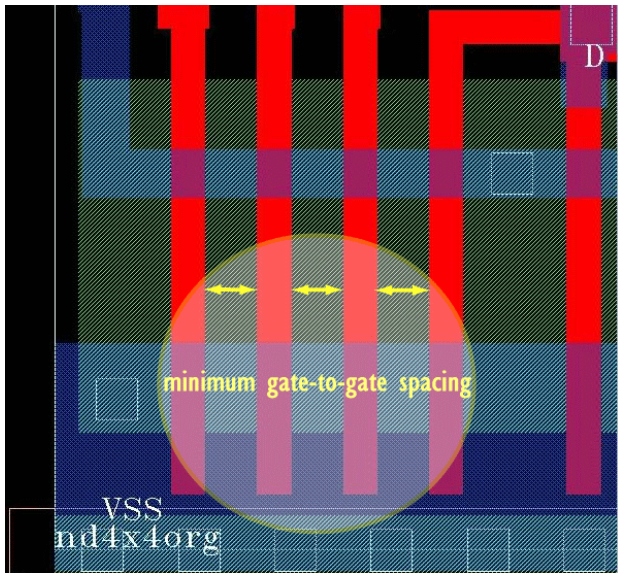
Figure 6. Minimum gate to gate spacing
